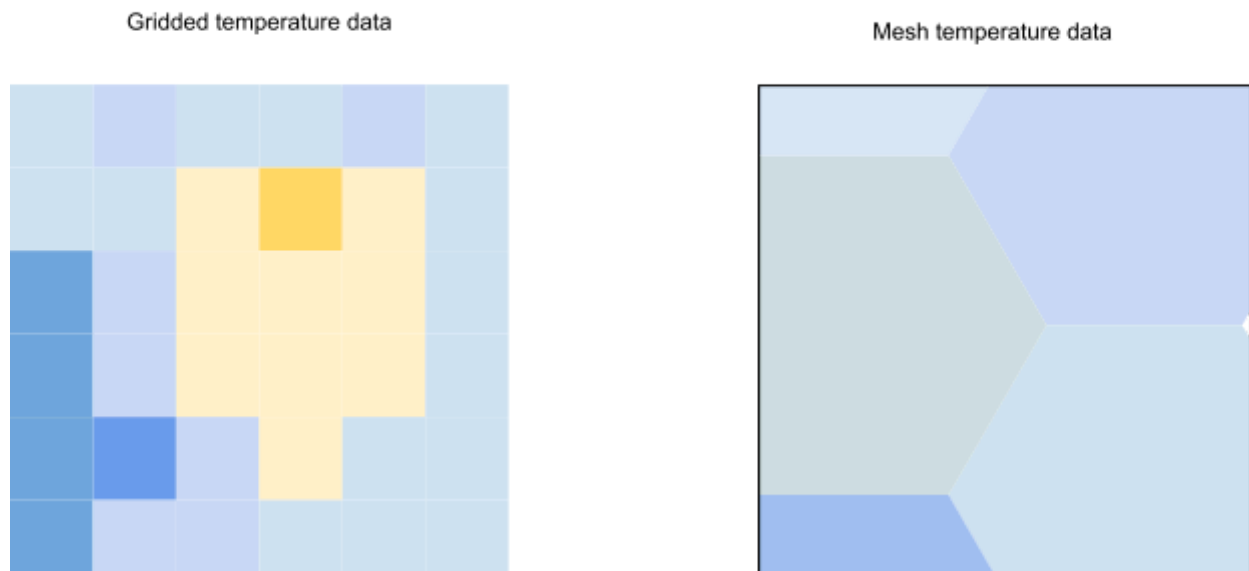
(Figure 31, original) Figure showing two temperature maps, one on a gridded system and one on a mesh system and how a cell of warm air is not visible on a gridded system.
